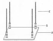
2. Place the Top Shelf (A) upside down on a flat & soft surface, and then lift it a little bit at one coner and insert 1 screw from the screw hole at the side of the bottom, then tighten one Connector (B) at the other side until secure. Repeat this step to secure all the other three Connectors (B) with the Top Shelf (A).
